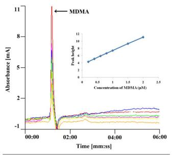
Figure 1. Calibration curve of the MDMA standard samples (concentration range:  $0.2-2 \ \mu g/L$ )
